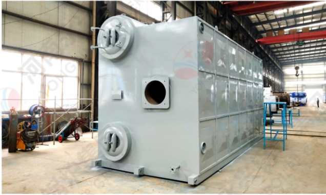
2018.10.23 蒙牛乳业（齐齐哈尔）15吨燃气蒸汽锅炉 2018.10.23 15t/h gas fired steam boiler in Meng Niu Dairy group (Qiqihaer)
